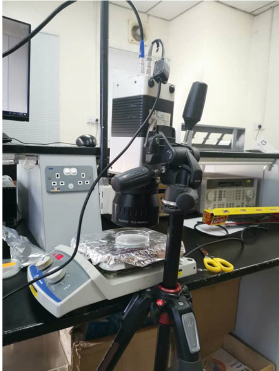
Fig. 2 Experimental setup for melting and solidifying process using thermographic camera
