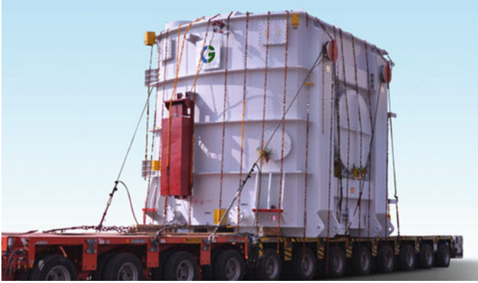
Fig. 2 A 1200 kV autotransformer manufactured by Crompton Greaves Ltd. [2]
