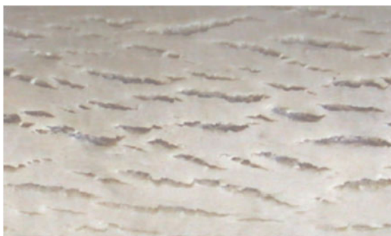
Fig. 7.5 Ozone images of SBR rubber after exposure of 4 h
