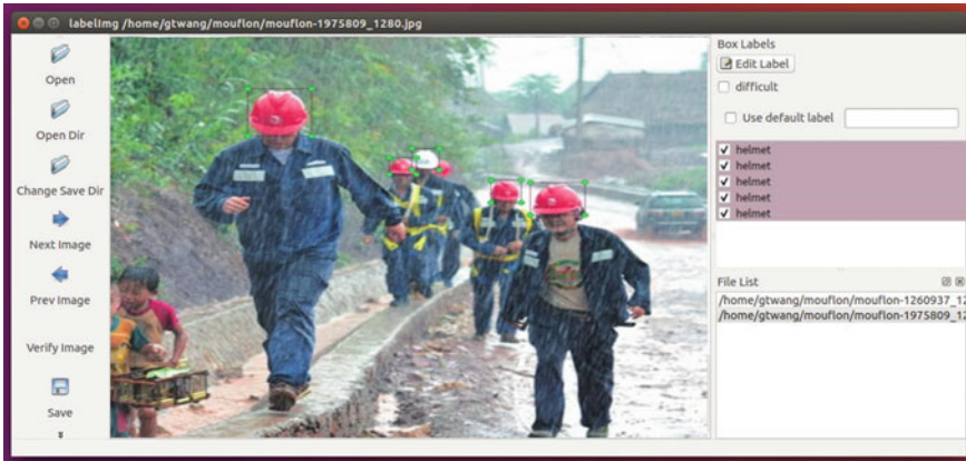
Fig. 6 Annotating image using the open-source LabelImg tool
