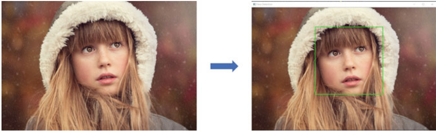
Fig. 8 Result of face detector module on an image
