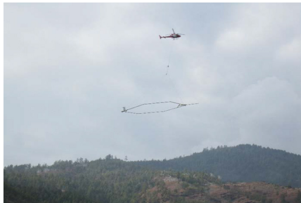
Figure 6. Performing geophysical surveys (AEM) along the tunnel alignment in hilly terrain in Bhutan
