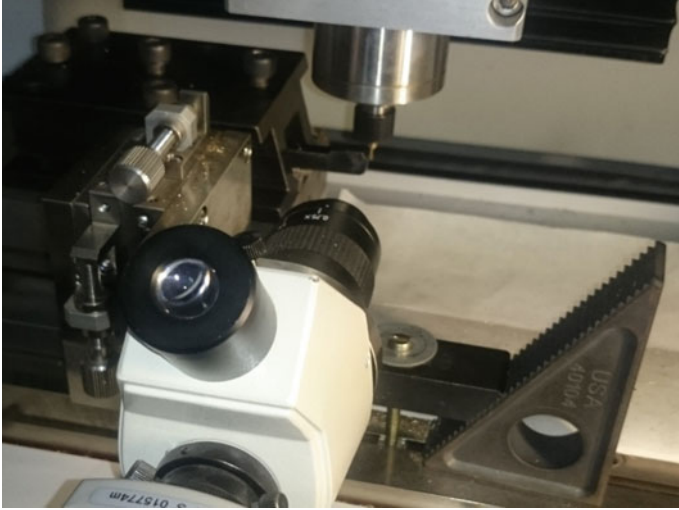
Fig. 1 Micro turning setup with WC insert
