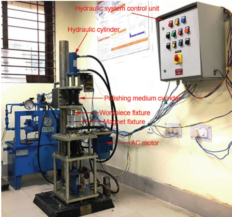
Fig. 12 Photograph of R-MRAFF experimental setup (micromachining laboratory, IITG)
