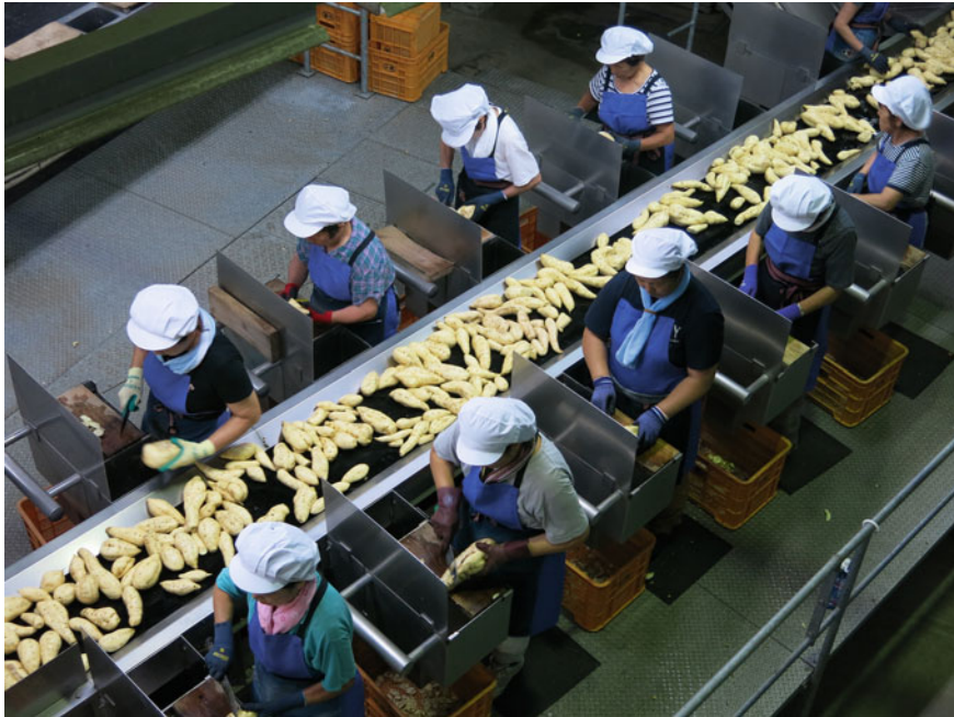
Fig. 5 Screening sweet potato in the shochu distiller. (Taken by the author, August 2013)
