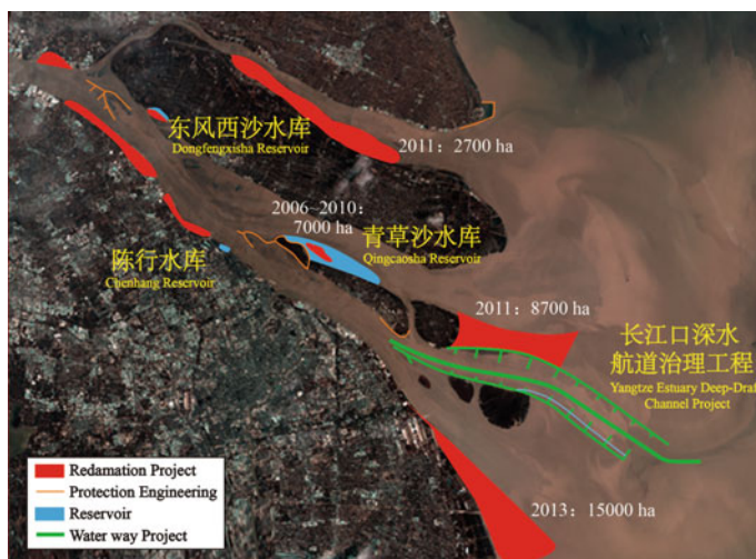
Fig. 2 Locations of engineering projects in the Yangtze River Estuary in recent years, including the development of the Qingcaosha Reservoirs and the Yangtze Estuary Deep-Draft Channel Project
