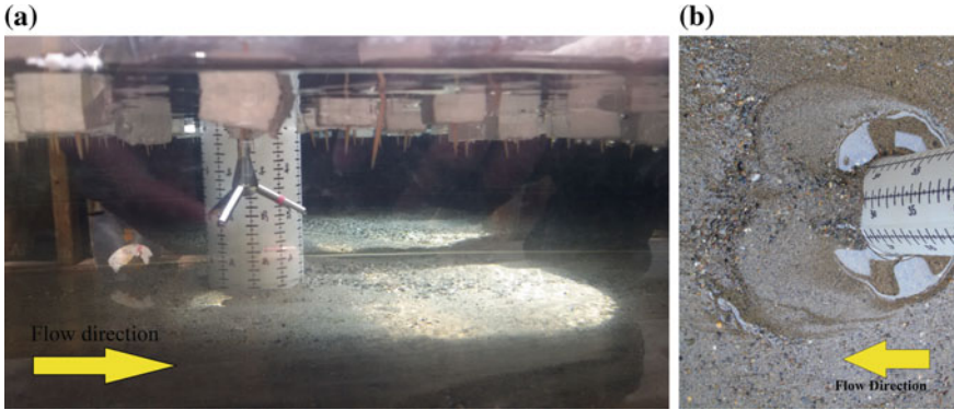
Fig. 2 a Side view of scour hole around the 11-cm-bridge pier under rough ice-covered condition, b top view of the local scour pattern around the 9-cm-bridge pier under rough ice-covered condition ( D_{50} = 0.50 mm)
