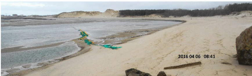
Fig. 4 Sand deposit behind the nets after several weeks
