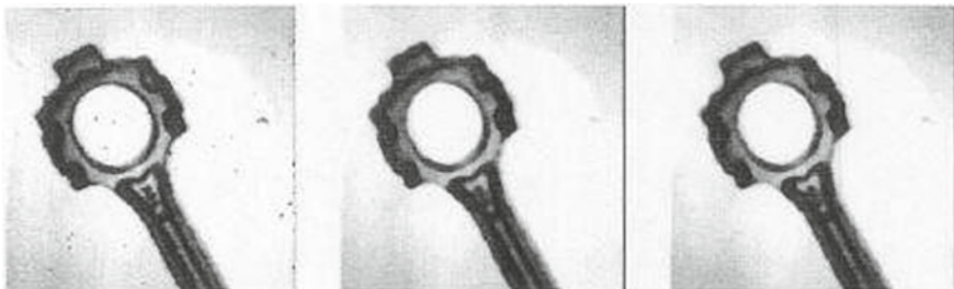
Fig. 8 Shows the results of a 3 \times 3 median filter on the corrupted images of Fig. 2
