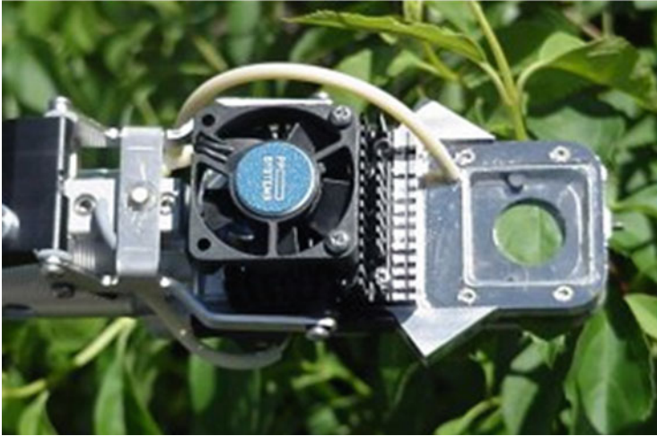
Fig. 3.2 Automatic universal leaf cuvette (Source: PP Systems, Massachusetts, USA)
