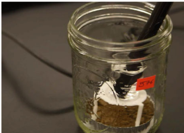
Fig. 12.1 Image of a respiration setup depicting the respiration trap inserted into the soil sample in a glass jar. The conductivity of the KOH is being read with an EC meter
