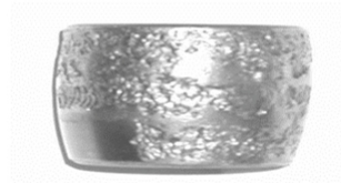
(b) Abnormal wear of rolling body
