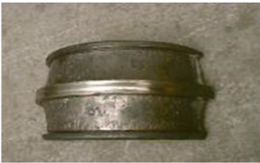
(a) Abnormal wear inner ring of bearing
