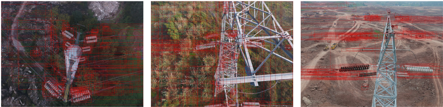
(c) Object detection result of RPN of Faster R-CNN(Fine-tuning anchors & PCA Jittering)
