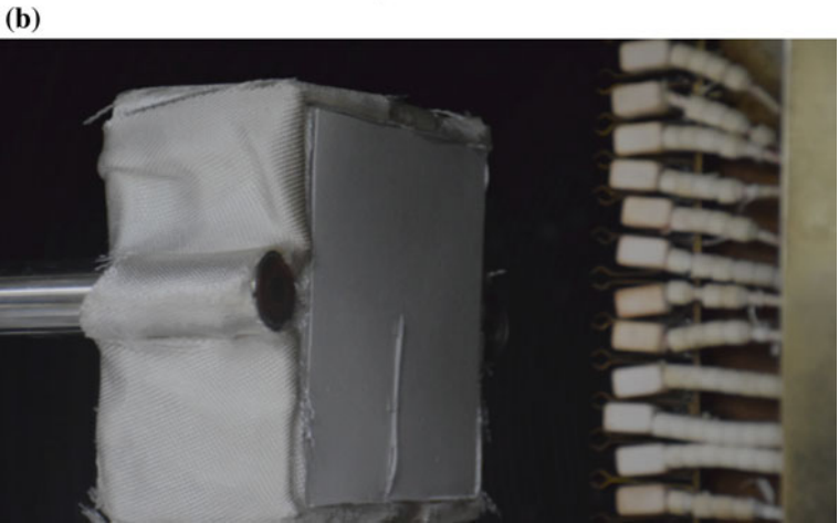
Fig. 2 a Schematic of instrumented specimen and b specimen mounted on a holder with heat flux sensor
