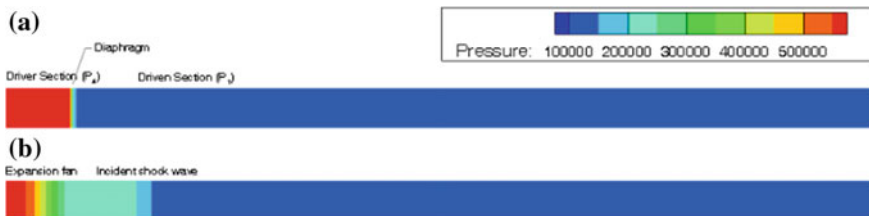
Fig. 6 Contours of pressure (in atm). a Initial. b After diaphragm rupture
