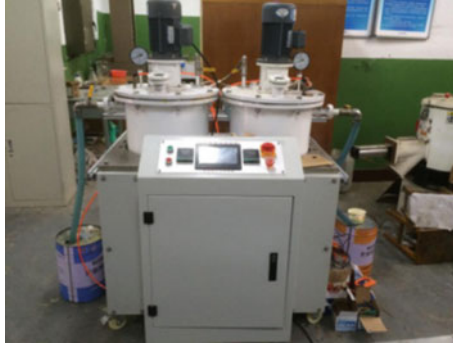
Fig. 1. Solventless laminating machine with vacuum defoaming function
