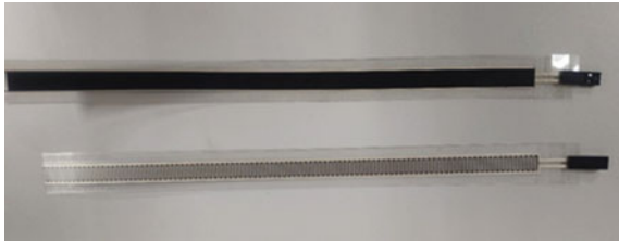
Fig. 2. Flexible bending sensor
