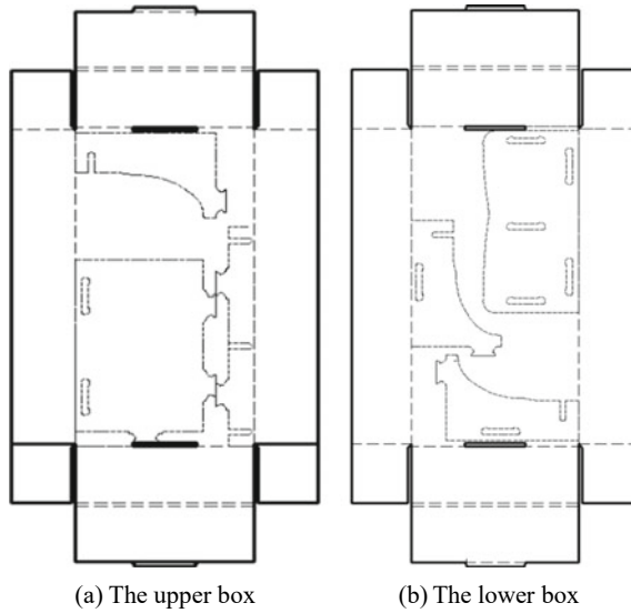
Fig. 1. Upper and lower expansion of packaging box
