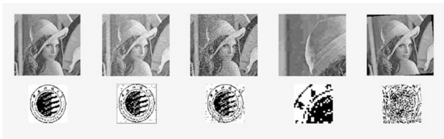
Fig. 4. The effects of digital watermark extraction after four attacks in DWT algorithm. Among them, a is the watermark image and watermark extract image of the DWT algorithm, b–e are the results of the images containing watermarks after applying Gaussian noise attack, pepper noise attack, cutting attack, rotating attack and the corresponding images watermark extraction
