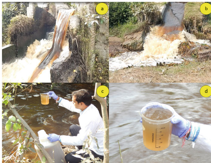
Fig. 1.1 Pulp and paper industry wastewater. (a–c) the huge volume of complex brown color wastewater generated during pulping and bleaching process and discharged into the environment after secondary treatment; (c, d) a large view of the collected pulp and paper industry wastewater
