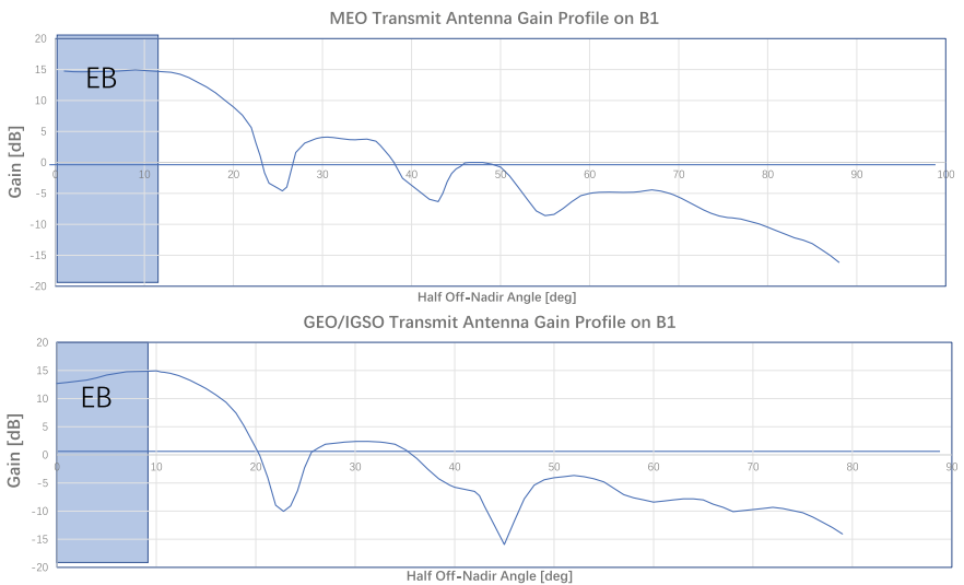
Fig. 3 Assumed BDS III transmitting gain for B1 versus off-nadir angle (EB represents blocked by Earth)
