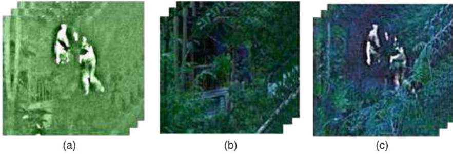
Fig. 14.2 An example scenario of video fusion of registered video streams: (a) an IR video sequence (b) a low-light visible video stream and (c) a fused video generated from (a) and (b)
