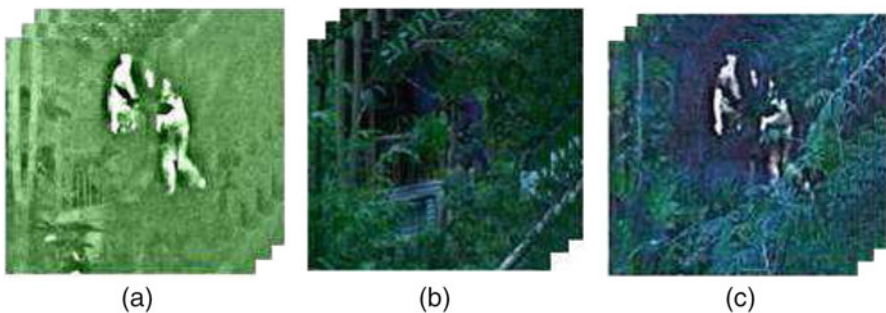
Fig. 12.1 An example scenario of video fusion of registered video streams: (a) an IR video sequence (b) a low-light visible video stream and (c) a fused video generated from (a) and (b)
