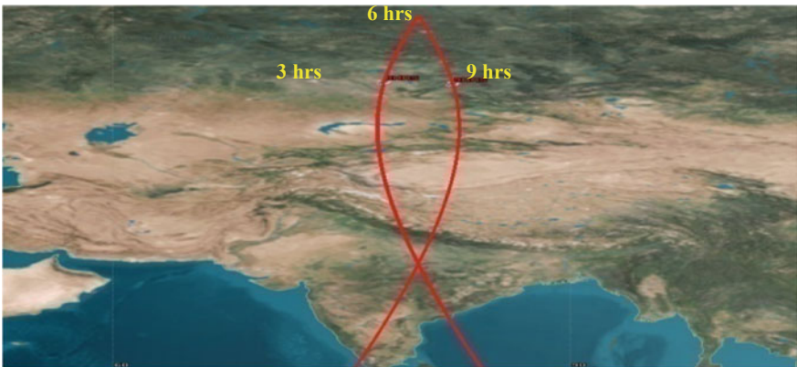
Fig. 4 Satellite subpoint at apogee \pm 3 h
