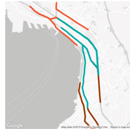
Fig. 4. Detected road communities in Thessaloniki, Greece. Each different color represents a group. Roads in the same communities varying together; in other words, travel times are more correlated. (Color figure online)
