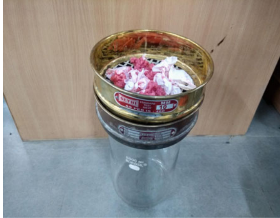
Fig. 4 Double sieve separation experimental setup using 10 mm top sieve and 1.18 mm bottom sieve
