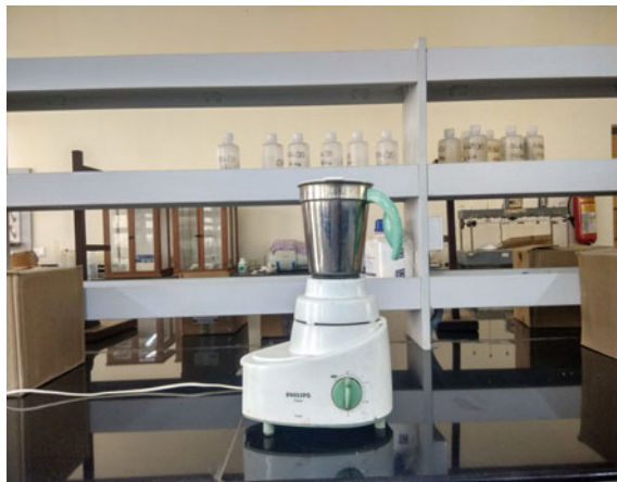
Fig. 2 Grinder system used to experiment with 750-ml jar volume and 186 grams of absorbent hygiene waste
