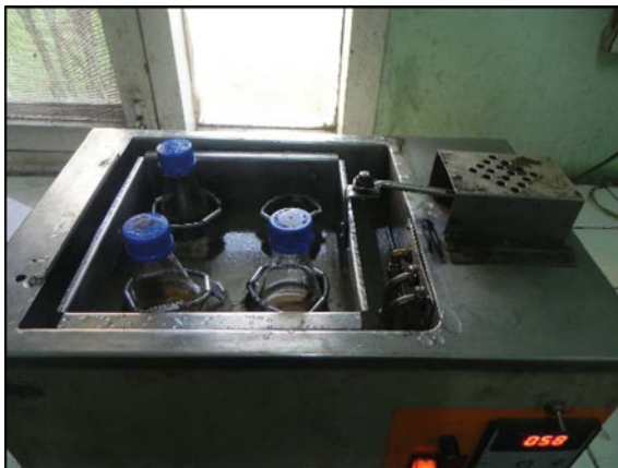
Fig. 1 Biodiesel production in water bath shaker
