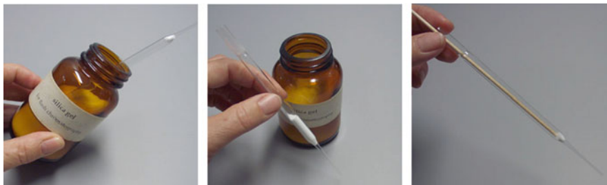
Fig. 13.2 Schematic representation of dry packing of column
