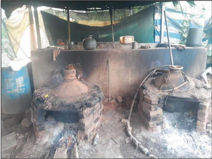
Plate 6.4 Bhann employed for distillation and collection of distillate
