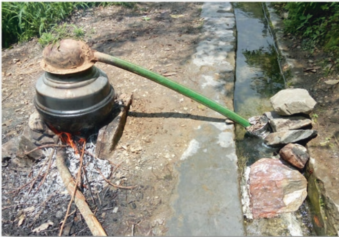
Fig. 22.4 Picture showing the arrangement used by Bhotiya community for distillation of Kacchi, an alcoholic beverage
