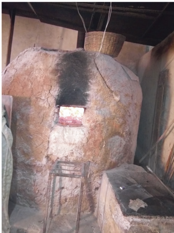
Plate 6.3 (a) Goan mud oven fired with wood used for baking “pao,” “kazara-bollo”
