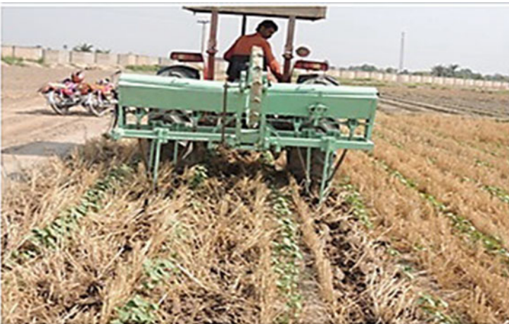
Fig. 16.2 Description of mechanical interculturing to incorporate wheat stubbles in relay intercropped cotton
