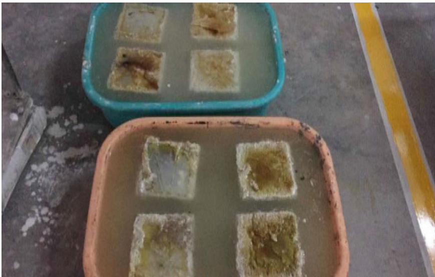
Fig. 11 Specimens in HCL and H 2 SO 4 after 28 Days
