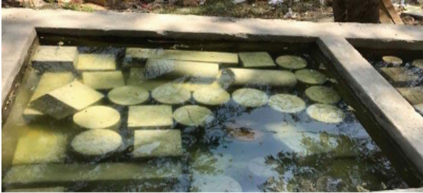
Fig. 7 Specimens in curing tank
