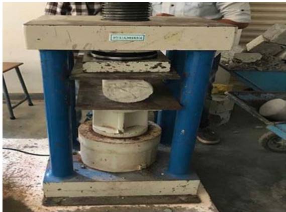
Fig. 9 Specimen under split tensile strength test
