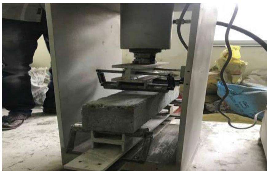
Fig. 10 Specimen under flexural test
