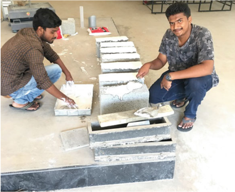
Plate 4 Capping of blocks before compression test
