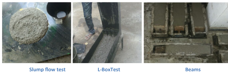
Fig. 1 Preparation and casting of specimens
