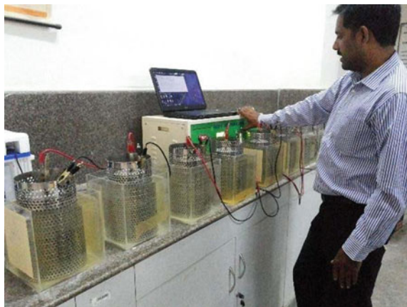
Fig. 2 Test setup for ACPT rapid chloride permeability test
