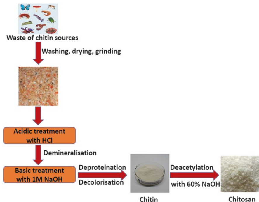
Fig. 11.7 Extraction of chitosan
