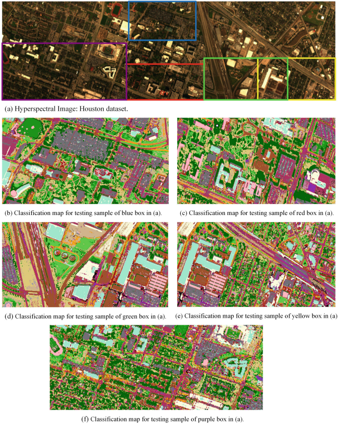
Fig. 4. Classification map obtained using the proposed method on Houston dataset. Here, boxes with different colors indicate the testing samples and its classification maps are displayed in (b)–(f).
