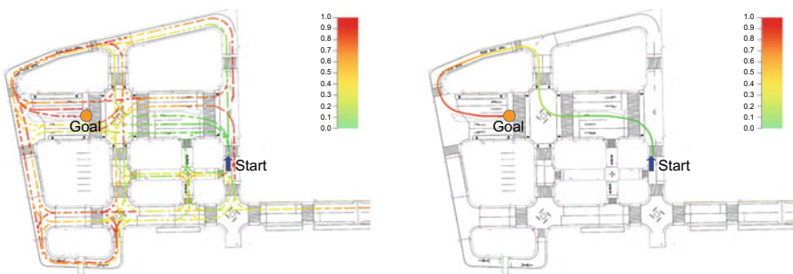
Fig. 4 Searching the map for the shortest path. Line color indicates route cost. Cost is represented by distance; green color is the closest distance to Start and red color is the max distance reached at the Goal position
