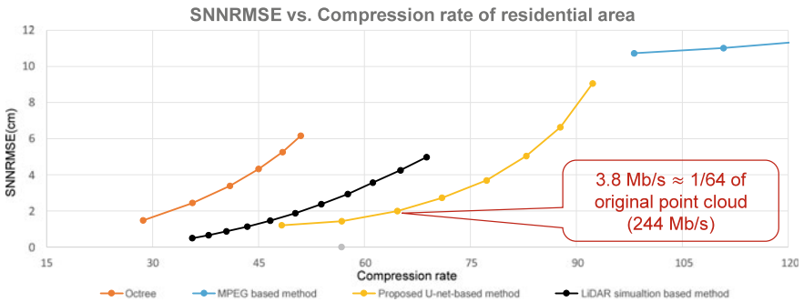
Fig. 7 SNNRMSE versus Compression rate for proposed U-net-based streaming point cloud compression method, in comparison with other compression methods. Symmetric Nearest Neighbor Root Mean Squared Error (SNNRMSE) is to measure loss after decompression
