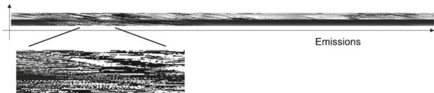
Fig. 3 Visualization of raw LiDAR packet data in an image-like format. A pixel's grayscale value from black to white represents a distance from 0 to 13,000 cm. Noted that without calibration, we could not understand this raw data in the way one understands a depth map
