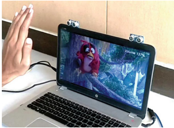
Fig. 10 Analysis of gesture use to control the volume of laptop and open the video clip
