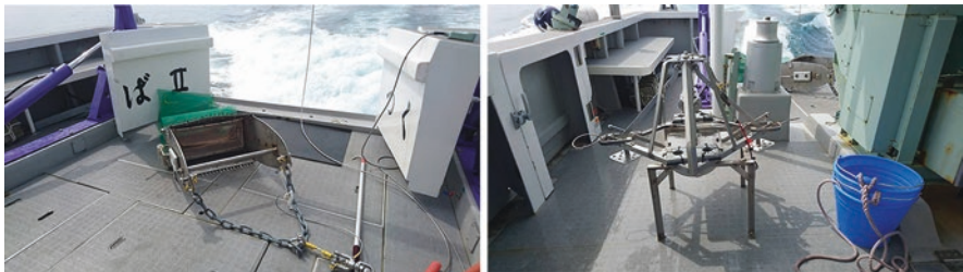
Fig. 22.5 Example of dredge, and grab sampling
