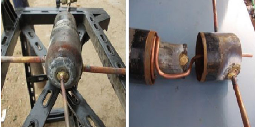
Fig. 1 Fabrication of low-pressure receiver
