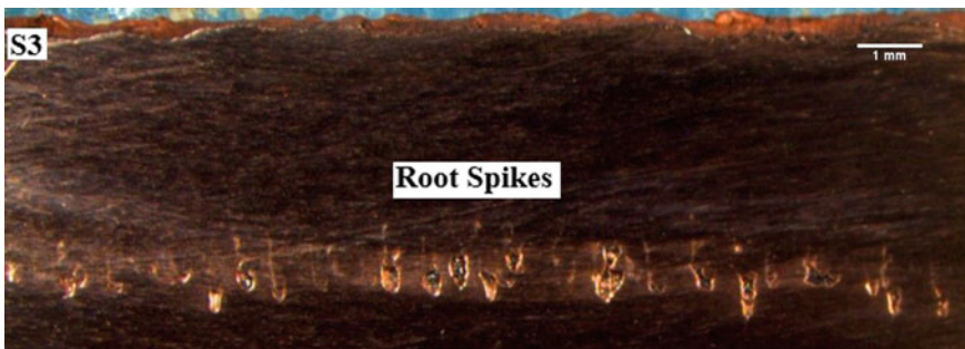
Fig. 3 Root spiking in electron beam welded copper plate (S3)
