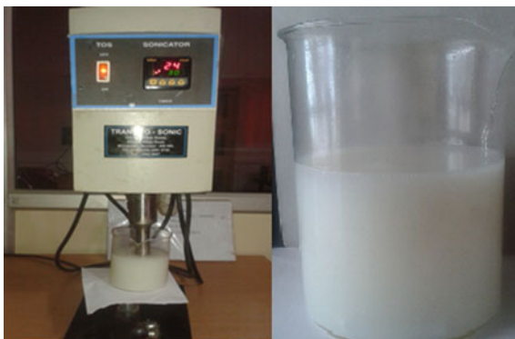
Fig. 4 Trans-o-sonic sonicator and prepared \text{Al}_2\text{O}_3 in POE nano-lubricant having weight concentration of 0.9 wt%
