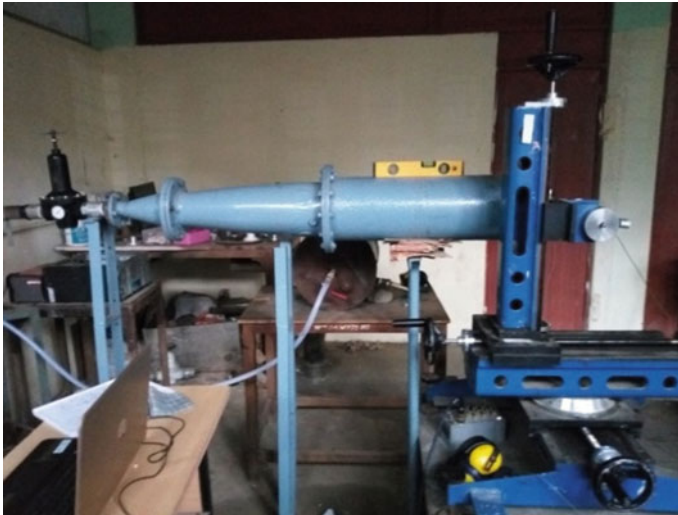
Fig. 2 Photographic view of the high-speed jet facility
