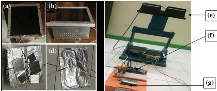
Fig. 5 a Top view of hybrid system, b Side view of hybrid system, c Connection of TEGs, d PV cell attached with aluminum foil, e Solar simulator halogen light, f Voltage, current, and temperature sensors connected to Arduino Uno, g LCD Display
