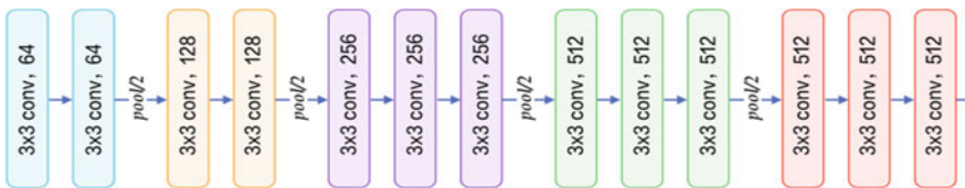
Fig. 5 CNN layer structure of VGG-16 architecture. Kernel size and number of neurons are denoted in each layer
