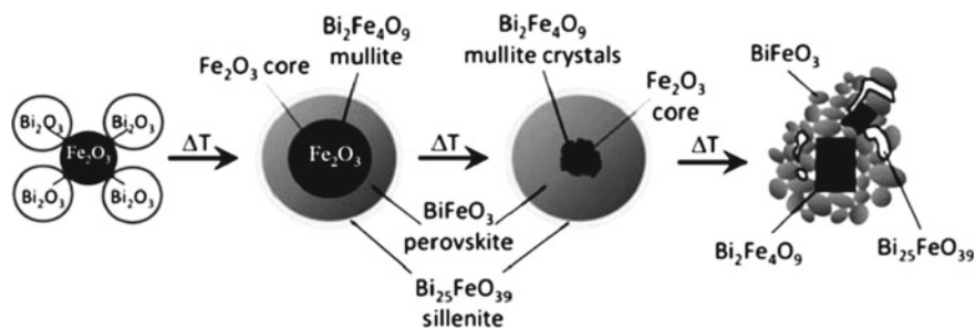
Fig. 3 A schematic diagram illustrating the reaction paths in the solid-state synthesis of BiFeO 3 . When the solid-state reaction proceeds, the penetration profile of the Bi ions into the Fe 2 O 3 particles leads to the formation of different compounds. Initially, the 25:1 (Bi:Fe) sillenite phase is formed in the outer surface and the 1:1 BiFeO 3 perovskite phase is developed as moving inside the structure. But the nuclei of the 1:2 Bi 2 Fe 4 O 9 phase is also formed in deeper inside, constituting the diffusion/reaction front toward the iron oxide core. As the temperature increases diffusion will be favored and more perovskite may be formed in spite of the iron-rich nucleus. Due to the competition between the complete formation of BFO and the crystallization of Bi 2 Fe 4 O 9 mullite crystals, the formation of BFO is blocked and eventually three phases coexist simultaneously. Reproduced with permission from [20], M. S. Bernardo, T. Jardiel, M. Peiteado, A. C. Caballero, M. Villegas. Reaction pathways in the solid state synthesis of multiferroic BiFeO 3 . J. Eur. Ceram. Soc. 31(2011) 3047–3053 Copyright © 2011, Elsevier Ltd.
