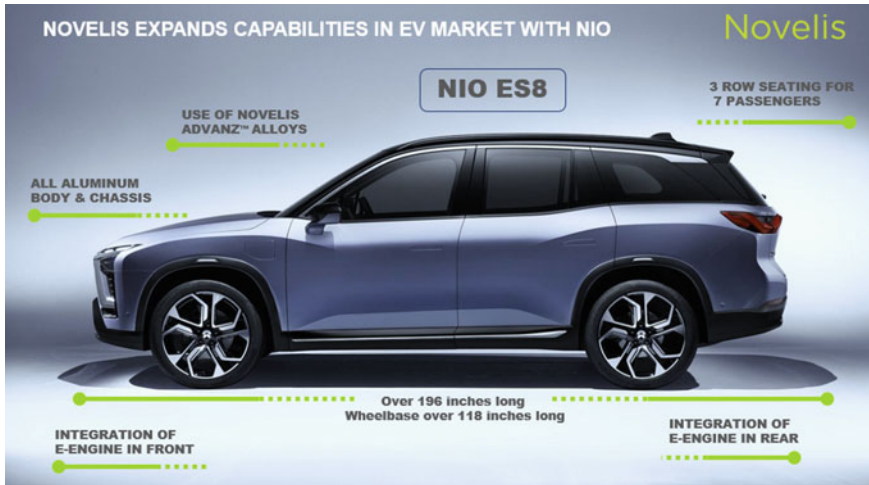
Fig. 3.9 New features in an electric vehicle NIO ES8, that use Al alloys extensively
