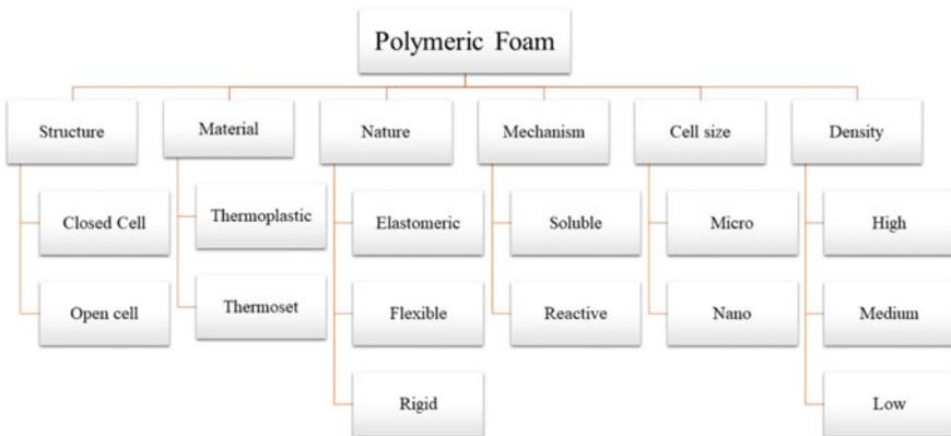
**Fig. 1** Classifications of polymeric foams based on different parameters
