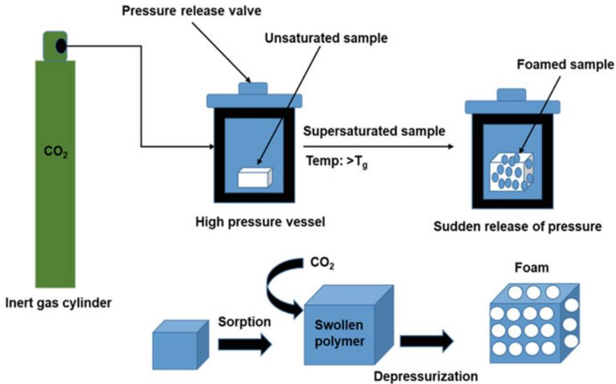
**Fig. 5** A schematic representation of batch foaming process
