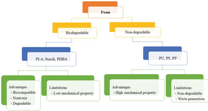
Fig. 3 Degradable and non-degradable foams
