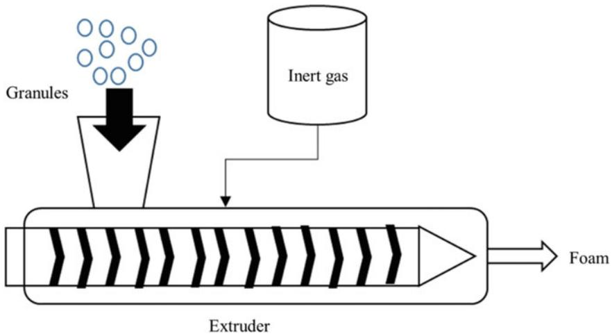
**Fig. 6** A schematic representation of continuous foaming process
