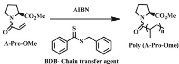
Scheme 2 General mechanism of reversible addition–fragmentation chain transfer polymerization (RAFT)
