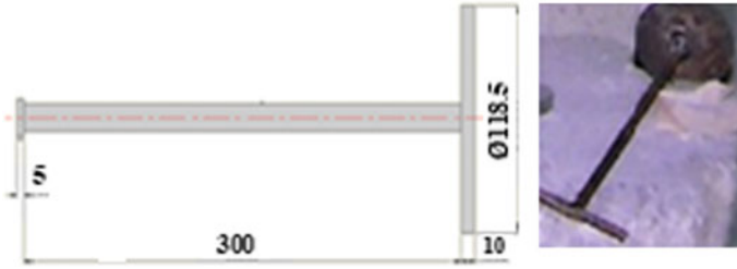
Fig. 2 Supporting door instrument design and fabrication
