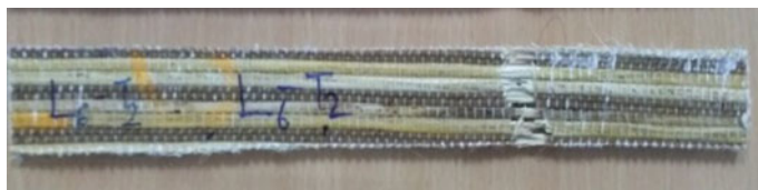
Fig. 1 Tensile test specimen failure mode
