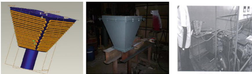
Fig. 4 Design (Left) fabricated prototype (middle) and testing set-up (right)
