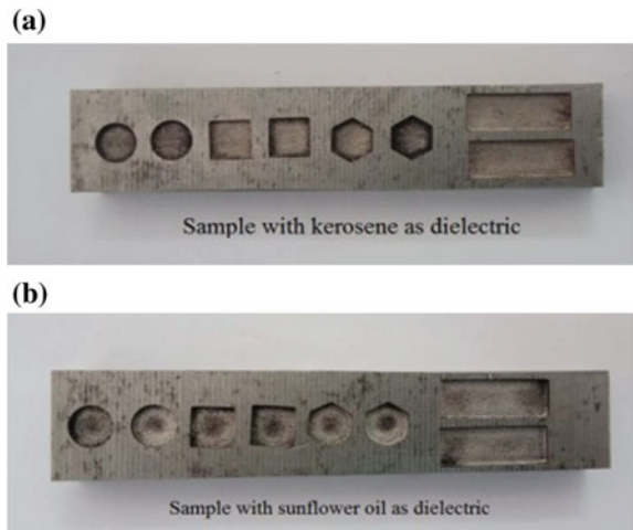
Fig. 3 a, b Machined samples a kerosene as dielectric fluid and b sunflower oil as dielectric fluid
