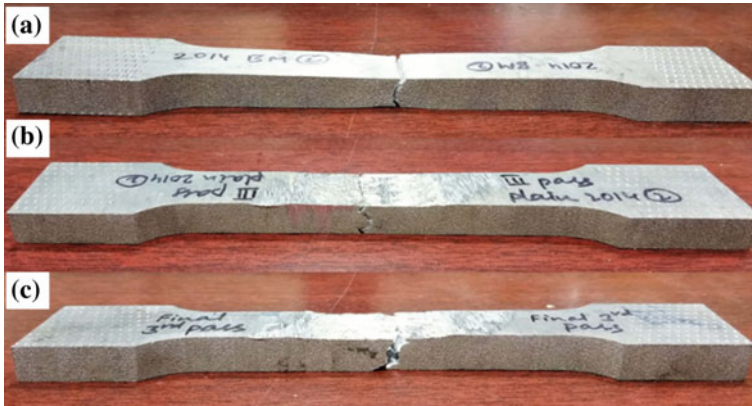
Fig. 9 Fractured lines after tensile test of a BM, b normal FSW joint c reinforced joint
