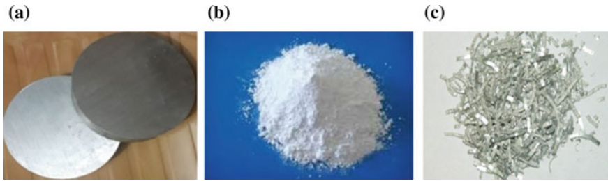
Fig. 1 a Al-7075 round bar pieces. b ZrO 2 in powder form. c Magnesium turnings
