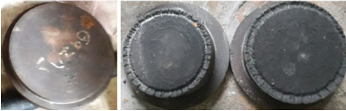
Fig. 3 Old die back door and its hot spot defect
