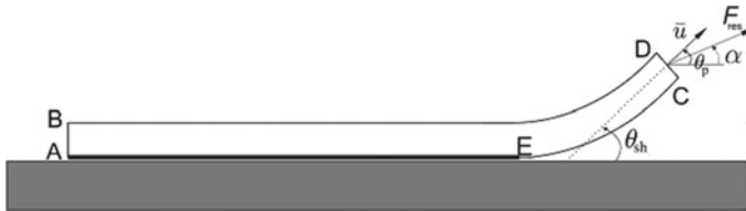
Fig. 2 Peeling by applied displacement
