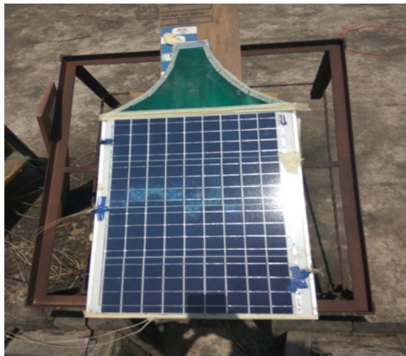
Fig. 1 Experimental set-up with PV/T collector
