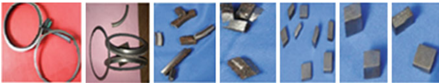
Fig. 5 Both old and new method cast castings rear side parting rings (chilled portion) can be made small pieces and its polished hardness tested specimens
