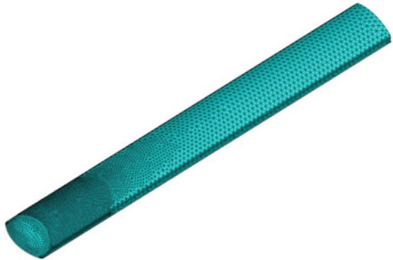
Fig. 3 Finite element mesh of wire tunnel segment-1
