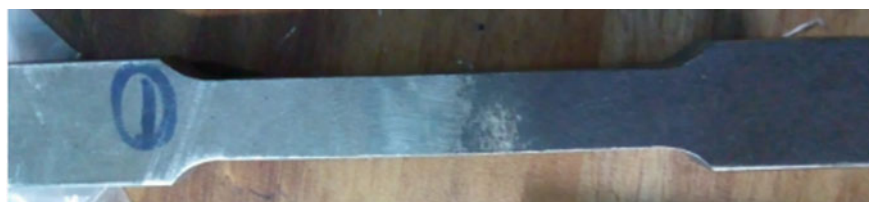
Fig. 3 Tensile test specimen (ASME SEC-IX: 2015)
