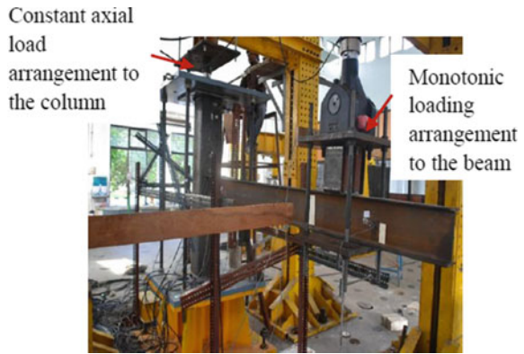
Fig. 4 Experimental set-up for mechanical loading to SHCWIB connection
