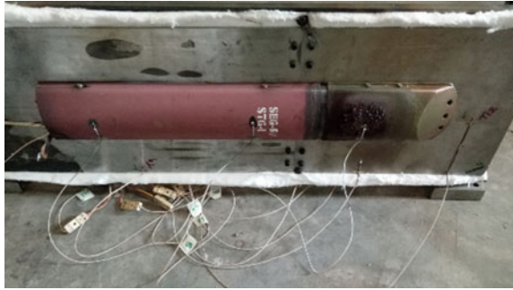
Fig. 12 Wire tunnel assembly after thermal test
