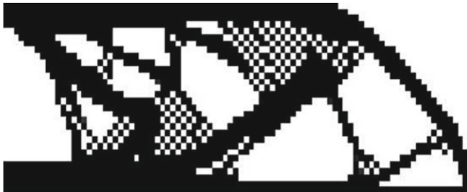
Fig. 2 Numerical effect of checkerboarding
