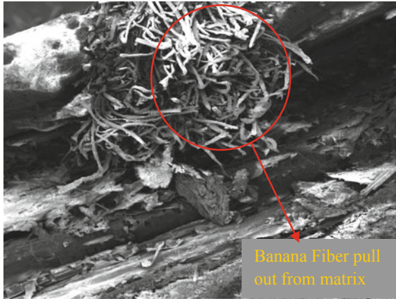
Fig. 19 Fiber pullout under loading
