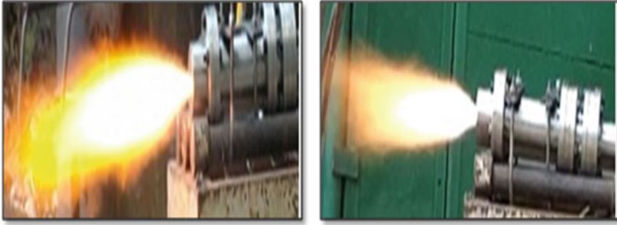
Fig. 6 Exhaust plume of bee-wax with and without VG with the pressure of 4.4 bar at t = 3 sec
