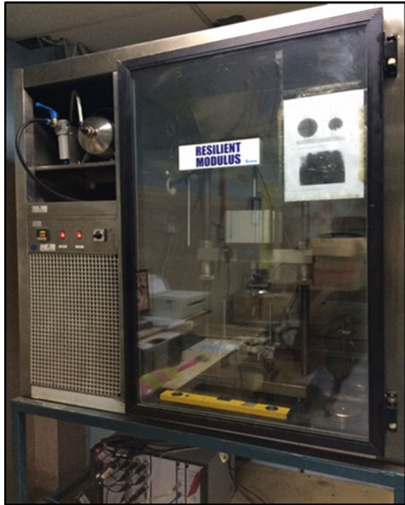
Fig. 3 The machine for indirect tensile modulus test
