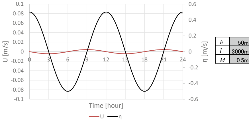
Fig. 4.6 Time series of tidal level \hat{\eta} and current velocity \hat{u} in Amitori Bay, as predicted using the theory of tidal flow dynamics in a single channel
