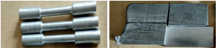
Fig. 5 Al 6082/SiC MMCs specimen with the addition of 10% SiC particulates
