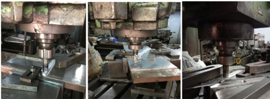
Fig. 3 Friction stir welding at weld angle 0°, 30° and 60°
