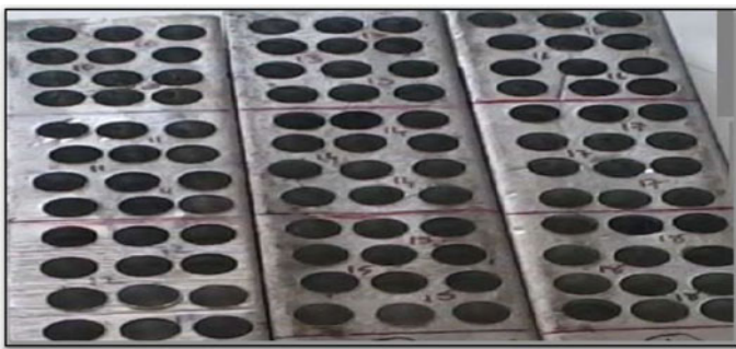
Fig. 2 Al6063–Al 2 O 3 MMC with 10, 15, and 20%
