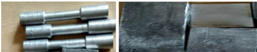
Fig. 2 Al 6082 specimen without the addition of SiC particulates
