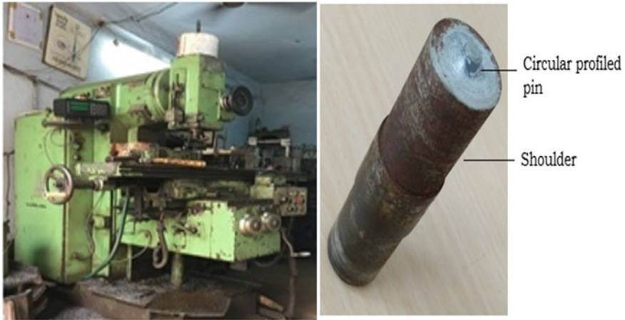
Fig. 2 Friction stir welding setup and circular profiled pin
