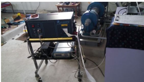
Fig. 7 Emission measuring instruments (AVL 437C Smoke Meter, AVL DIGAS 444 N)
