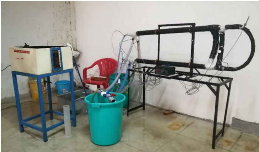
Fig. 1 Experimental setup of trio-tube heat exchanger
