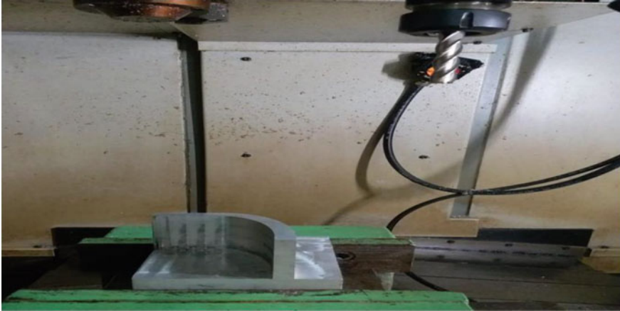
Fig. 6 Elliptical-walled part experimental setup
