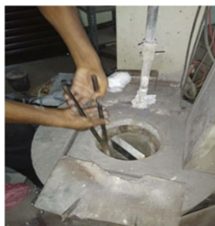
Fig. 5 Placing aluminum material in sand mould and heated the material up to 760 °C
