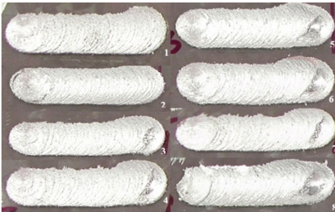
Fig. 4 Deposit of aluminium alloy over mild steel by the eight parameter combinations
