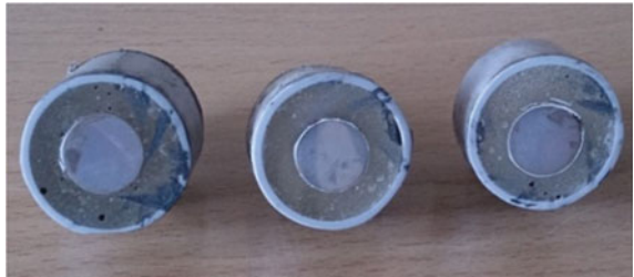
Fig. 6 Mounting samples of aluminum coating rods (without silica)
