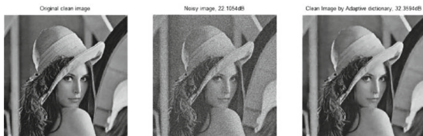
Fig. 4 Clean image, noisy image ( \sigma (standard deviation) = 25) and clean image by adaptive dictionary
