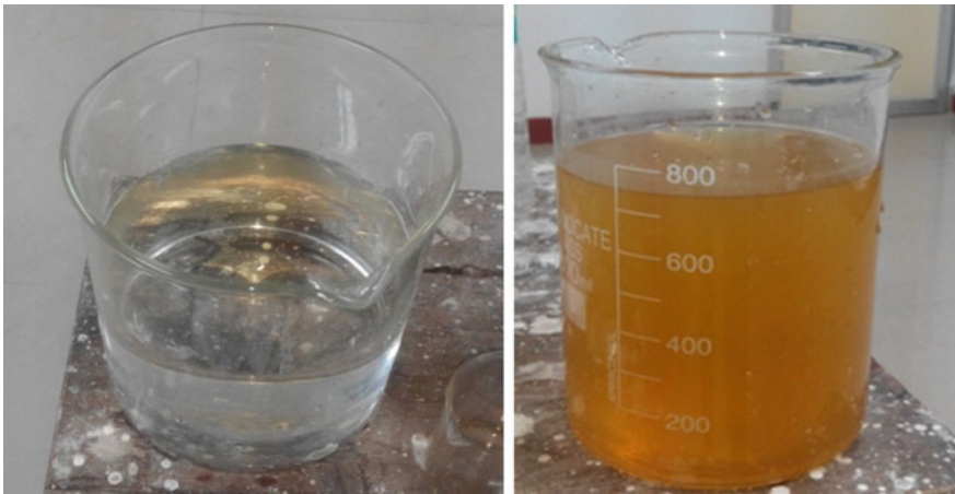
Fig. 4 NaCl electrolyte before and after machining
