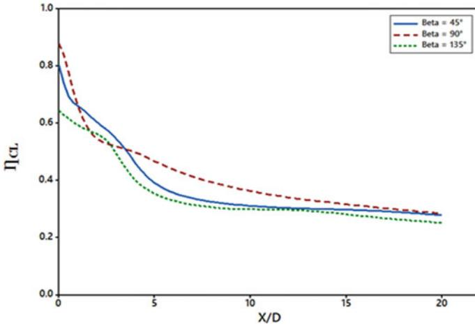
Fig. 5  $\eta_{CL}$  for different film hole compound angles at blowing ratio 1.2
