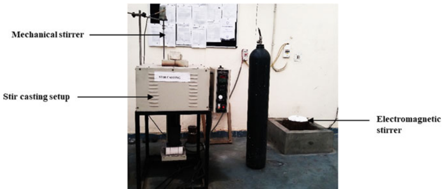
Fig. 1 Stir casting setup for composite fabrication
