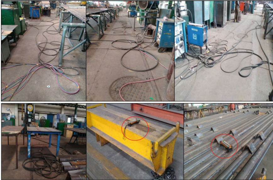
Fig. 3 Welding cable, air hose, oxyacetylene gas hoses and EOT crane remotes are placed in an unsafe condition
