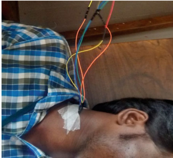
Fig. 5 Accelerometer sensor placement
