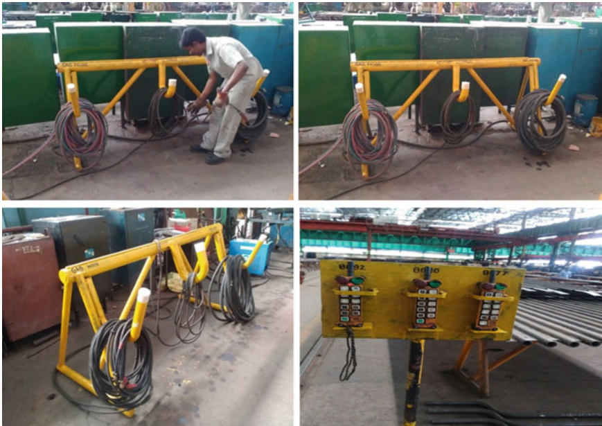
Fig. 7 Worker is placing the welding cable, air hose and oxyacetylene gas hose after completion of the work on the newly fabricated stand
