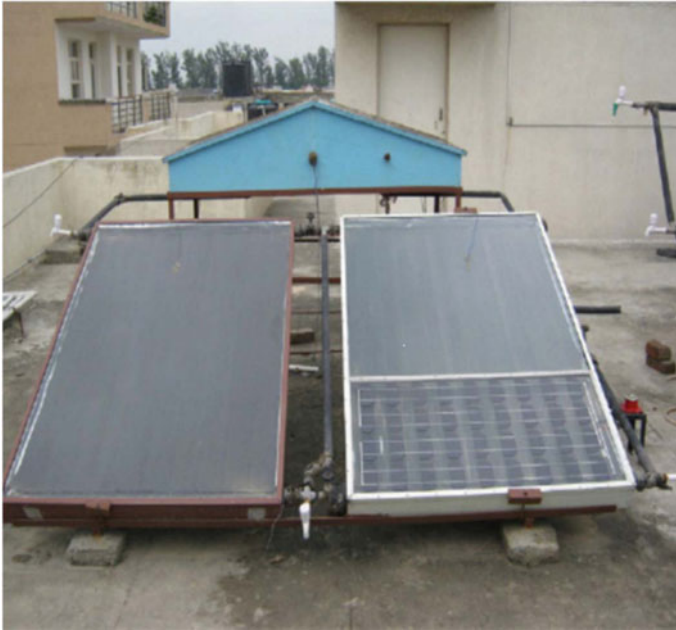
Fig. 2 Setup of double slope solar desalination unit integrated with two FPCs [9]
