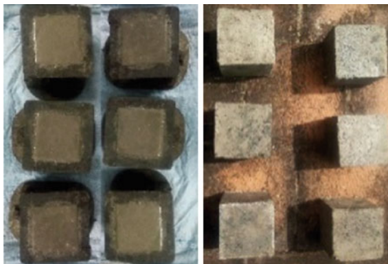
Fig. 26.1 Casting and curing of geopolymer concrete
