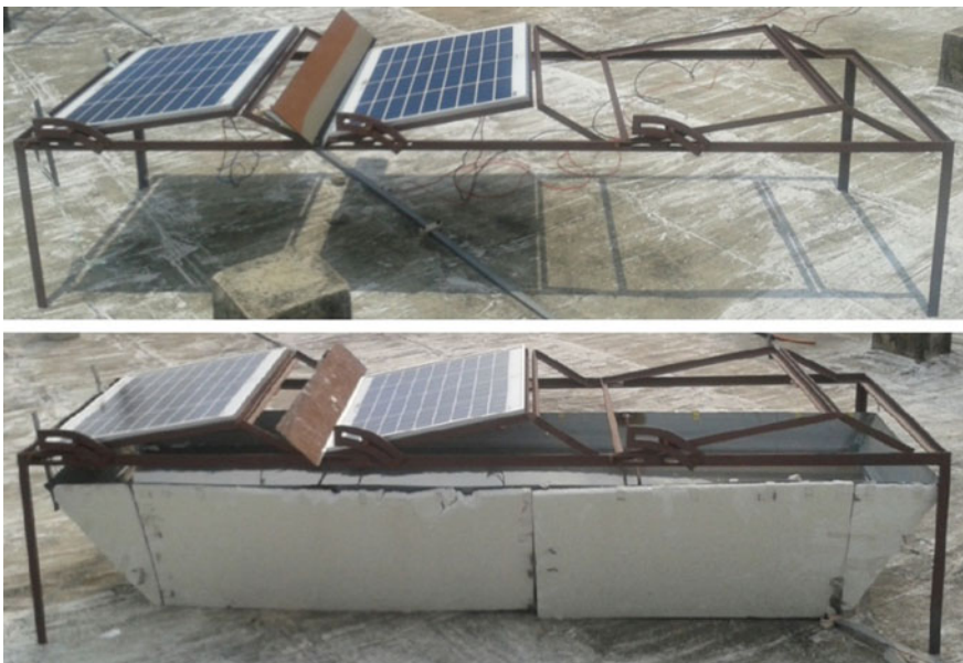
Fig. 8.5 Experimental setup for a ground-mounted system and a canal top system
