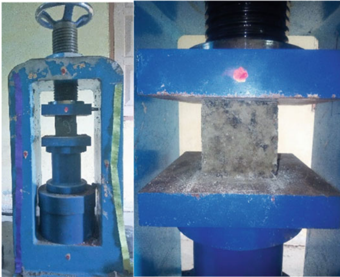
Fig. 26.2 Testing of concrete specimens
