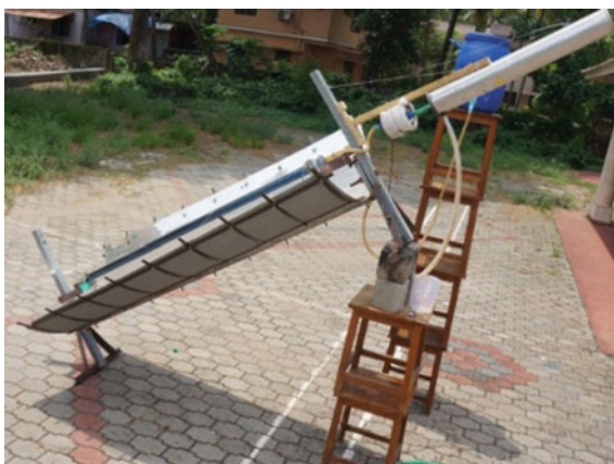
Fig. 20.4 Experiment setup using steam trap
