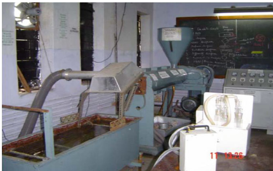
Fig. 6 Eco-friendly waste plastics process and machine developed and patented for producing recycled granules by Prof. S.K. Ghosh, at Jadavpur University, Kolkata
