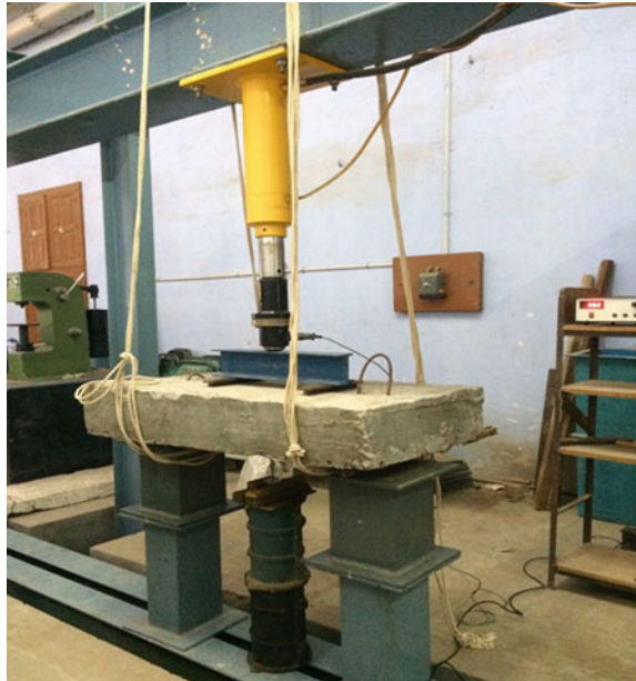
Fig. 4 Experimental setup of the slab
