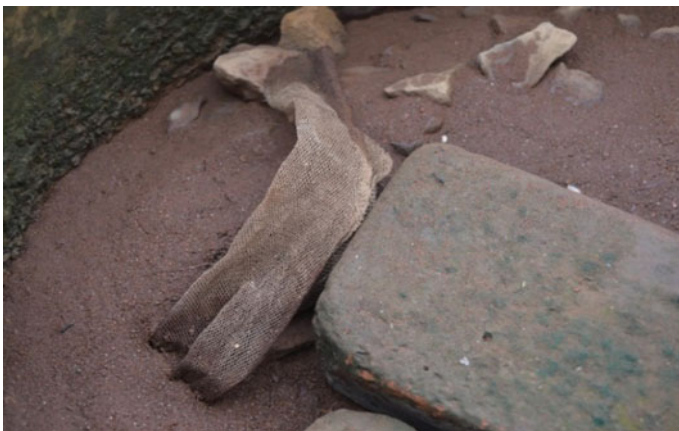
Fig. 3 Reddish layer formed on top of the filter media of the selected filter unit
